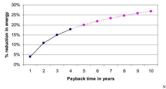
Figure 4 Potential reduction in industrial energy use from EE measures
